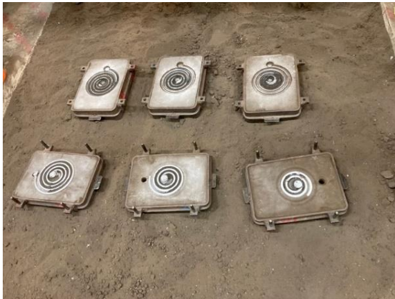
Fig. 3. Open mold showing the cast aluminum after solidification.
